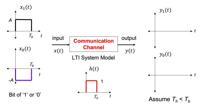
(a) Plot  $y_1(t) = h(t) * x_1(t)$ . Label the important points on the vertical and horizontal axes in terms of A,  $T_b$ , and  $T_h$ . Assume  $T_h < T_b$ . 4 points.
